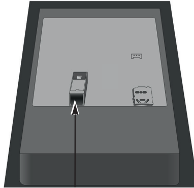
The RJ10 connector of the control cable is plugged into the control panel. The RJ14 connector is plugged into the power unit.
