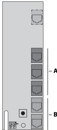
A RJ10 plug for sensor line B RJ14 plug from control panel
